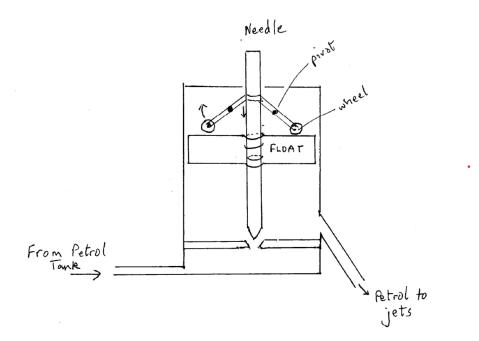
If the petrol-air mixture is wrong, it can be changed in one of two ways: changing the jet, or changing the height of the float.
